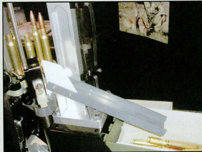
View of the ramp at position 5 that guides finished rounds into the ammo box. Photo © 2011 by Dale Arenson
