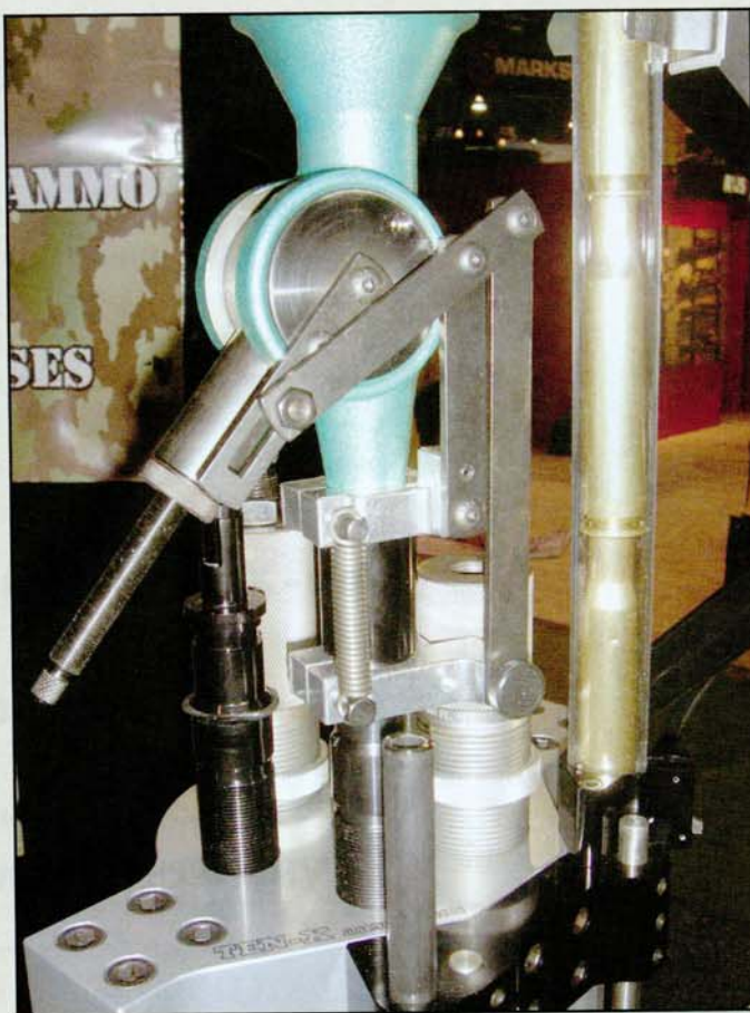
Tool head with dies, powder dispenser, and shell feeder tube at right. Primer feed tube in the foreground. Photo © 2011 by Dale Arenson
