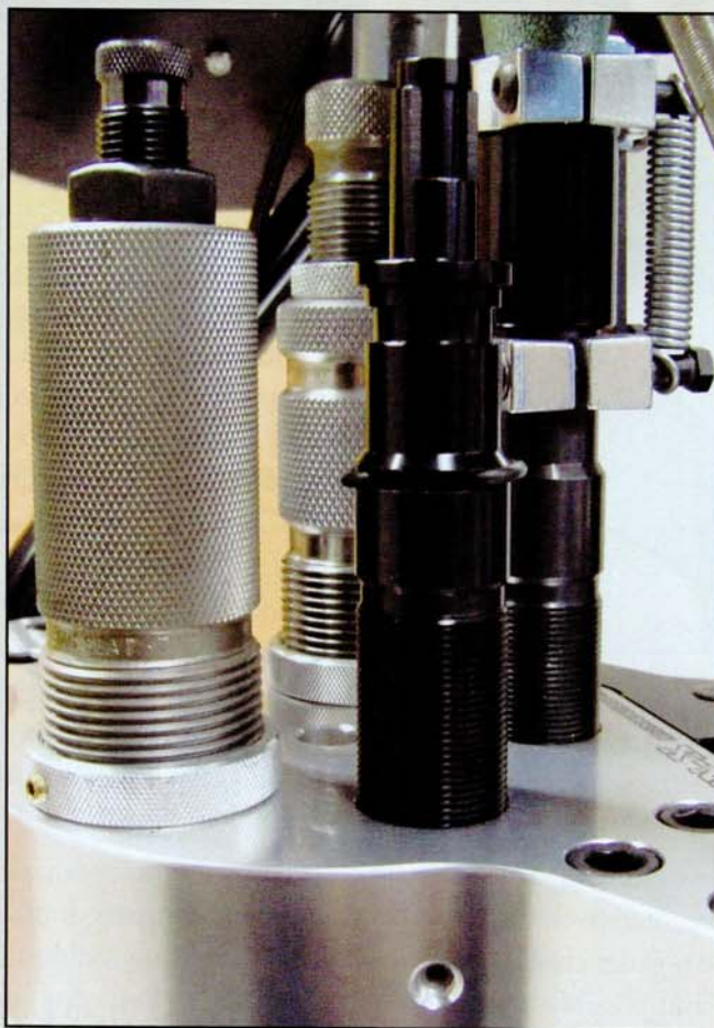
The powder check die at position three. Lock rings are not required because of the nylon set screw below the die.
