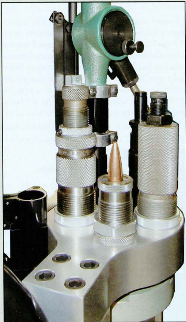
View from the rear of the tool head. Left to right, positions 1, 5 and 4 with sizing, crimping and seating dies. Photo © 2011 by Ten-X Ammunition
